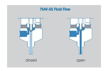
The primary control of deposit size is the valve open time.
